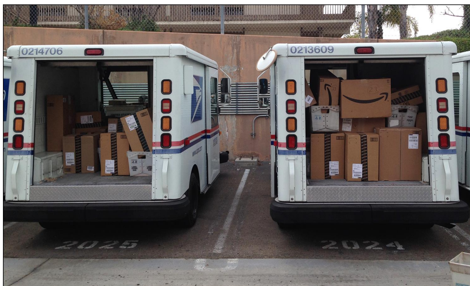
Figure 5: U.S. Postal Service Delivery Vehicles with Insufficient Loading Space to Accommodate Large Packages
