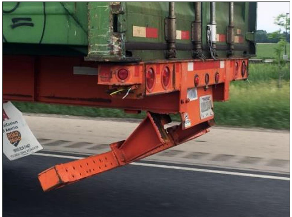
Figure 5: Example of a Damaged Rear Guard
