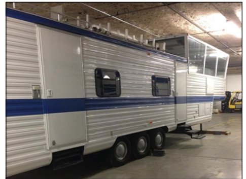
Mobile air traffic control tower at the Mobile Asset Deployment Center in Independence, Missouri
