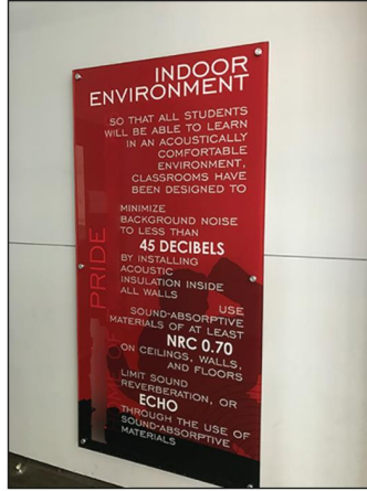
A sign in a California school explaining changes made during a recent renovation.
