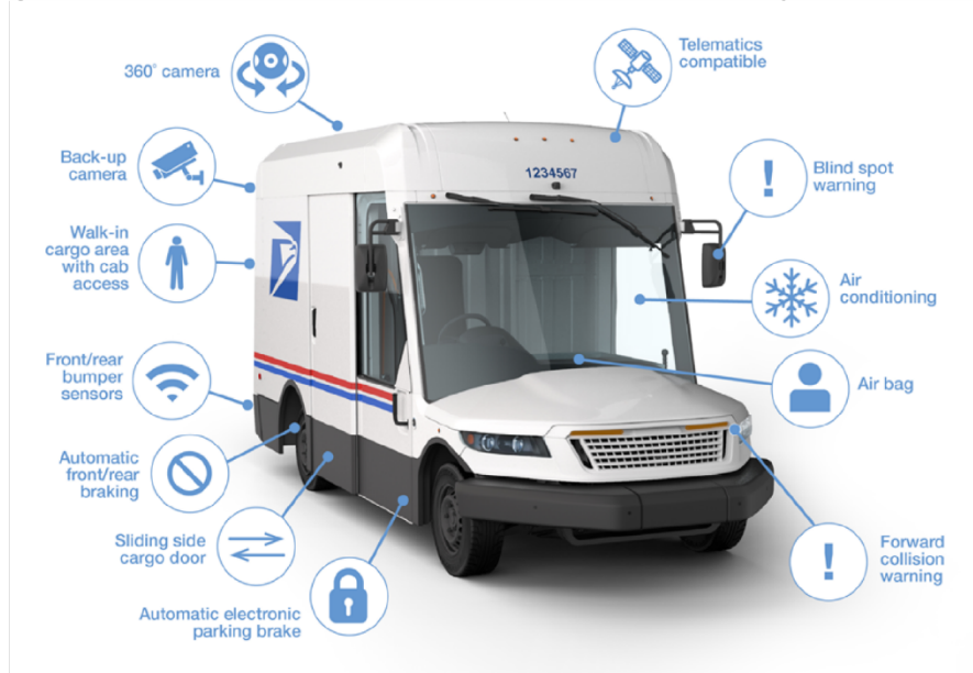
Figure 4: Concept Drawing of the U.S. Postal Service's (USPS) Next Generation Delivery Vehicle
