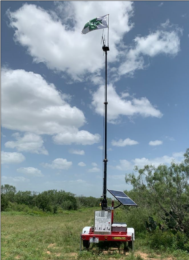
Figure 3: Rescue Beacon and 9-1-1 Placard Deployed Along the Southwest Border
