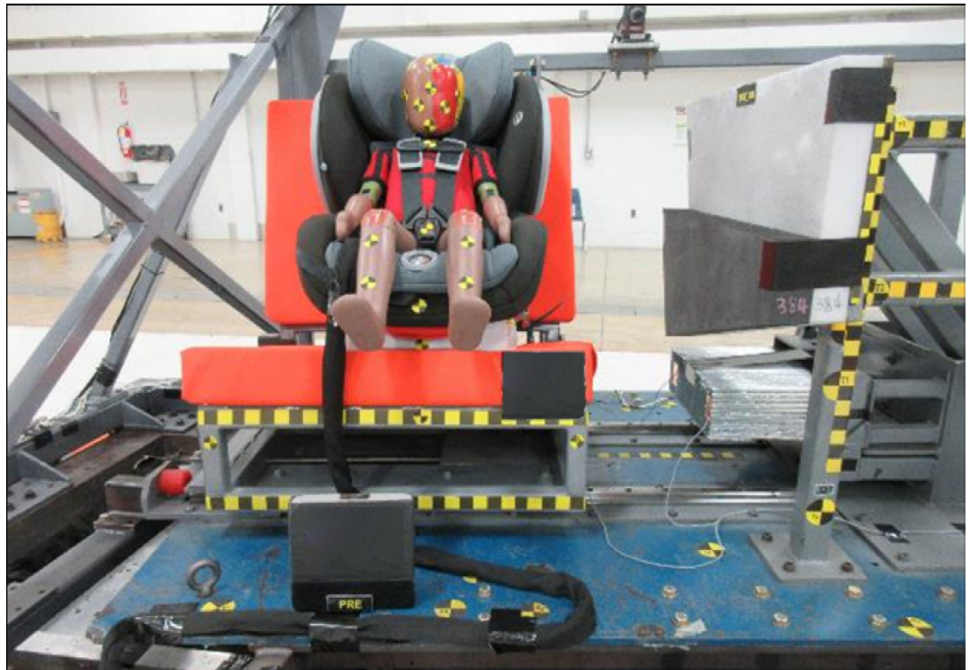
Figure 14: A Child Crash Test Dummy in New Side-Impact Sled Test
