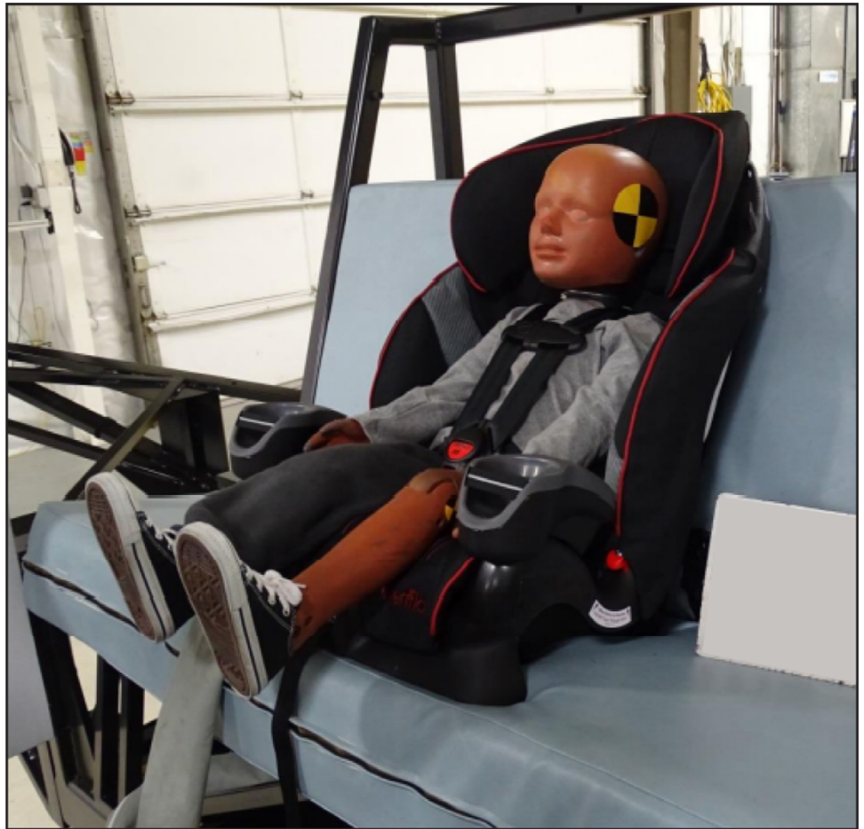
Figure 13: A 3-Year Old Child Crash Test Dummy in a Frontal Sled Test
