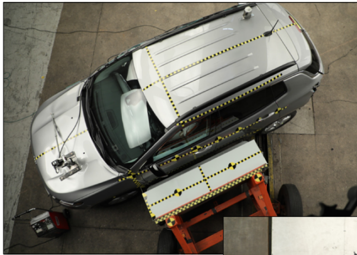
Side barrier crash test
