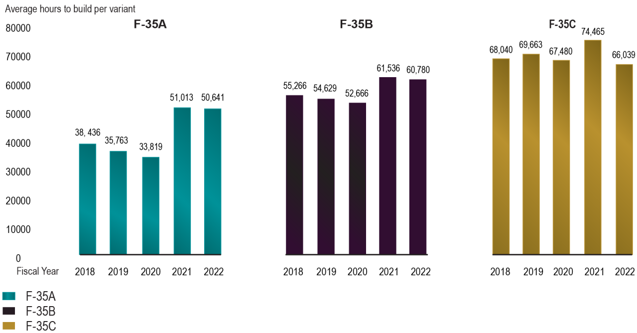
Figure 6: F-35 Aircraft Are Generally Taking Longer to Build in Recent Years
