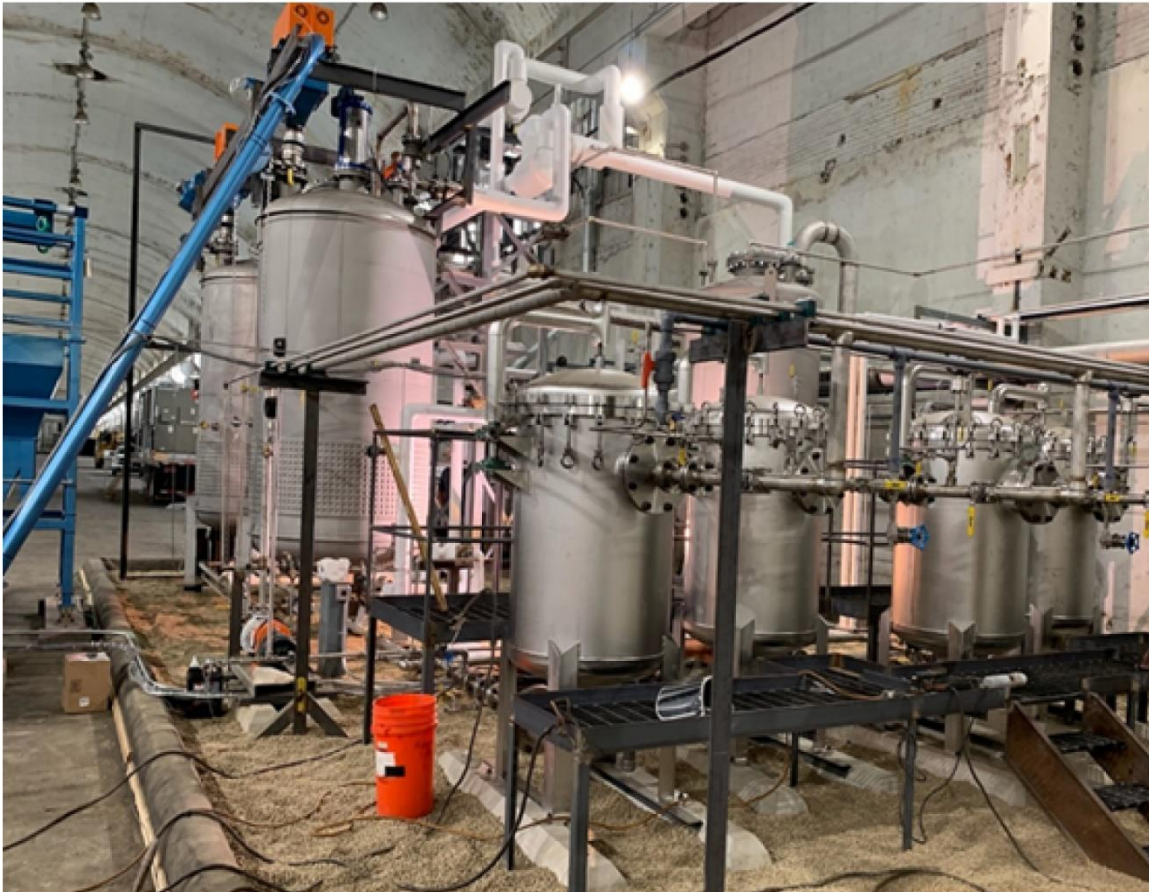
Figure 5: A pilot-scale facility in Pennsylvania for rare earth element extraction from coal ash
