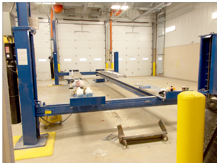
Figure 8: Exterior and Interior of Recently-Constructed Bus Maintenance Building Where Door Does Not Close When a Large School Bus Is On Hydraulic Lift
