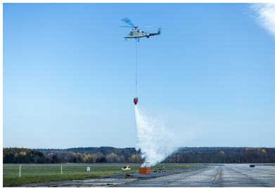
[An unmanned Lockheed Martin/Kaman K-MAX helicopter extinguishes several fires, aided by the small unmanned Indago Quad Rotor, also from Lockheed Martin, during a demonstration.]
