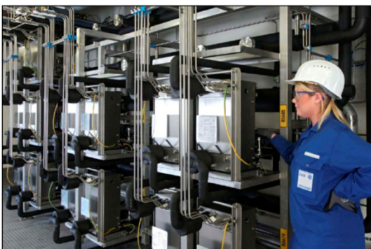
Figure 18: Continuous flow microreactors in a pharmaceutical production plant
