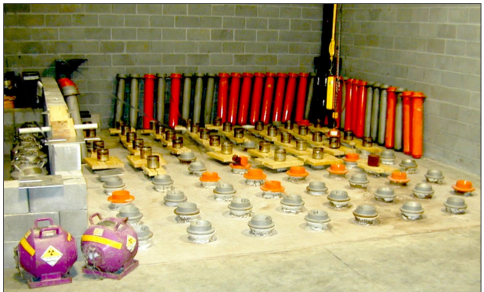
Figure 3: Well Logging Storage Facility with Multiple Containers for Storing Radioactive Material
