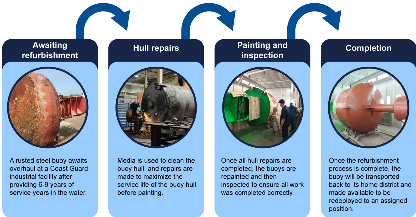
Figure 13: Summary of the Refurbishment Process for a Steel Buoy
