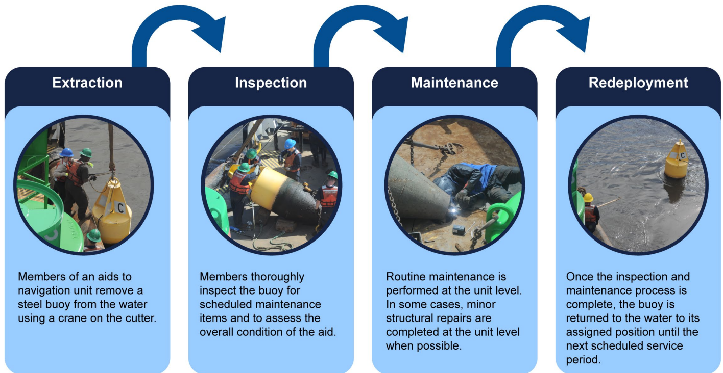
Figure 4: Process Used by Coast Guard Aids to Navigation Units for Servicing Steel Buoys
