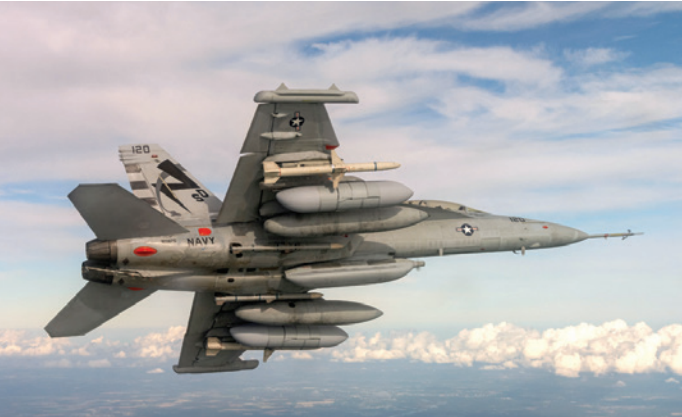
Next Generation Jammer Mid-Band (shown on an EA-18G Growler aircraft)
