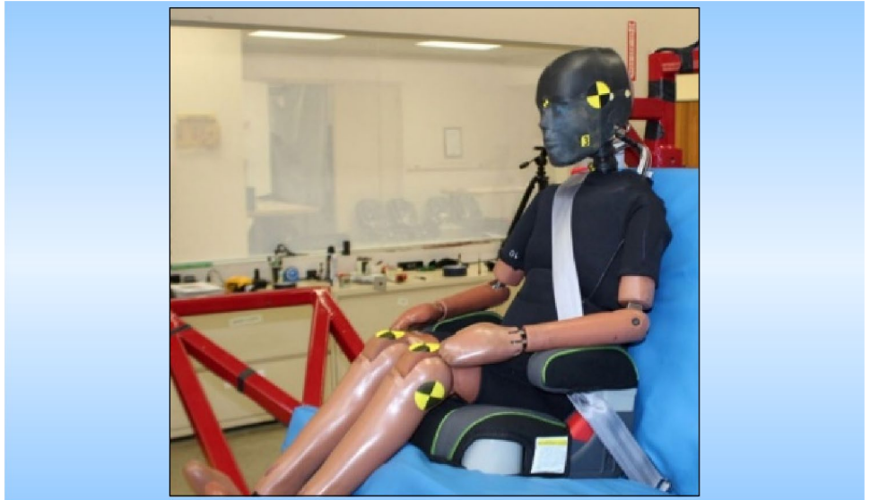
Figure 9: Development of the Large Omnidirectional Child Dummy
