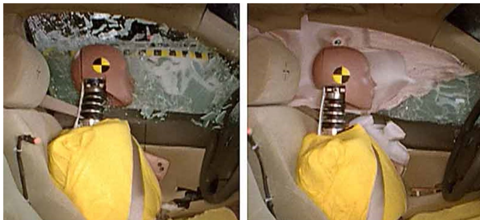
Figure 5: Side-Impact Crash Test, without and with a Side Airbag
