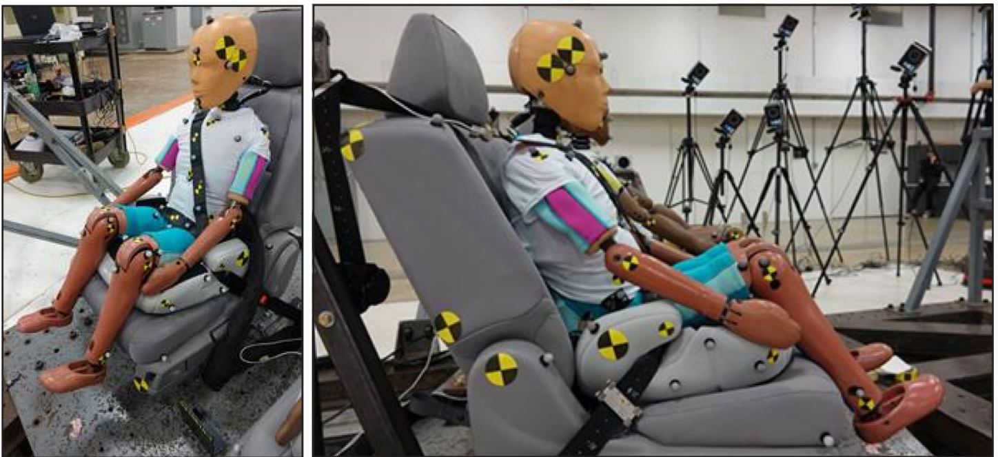
Figure 12: Large Omnidirectional Child Crash Test Dummy
