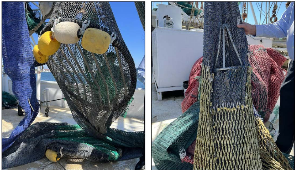
Figure 7: Turtle Excluder Device (TED) and Bycatch Reduction Device (BRD) on Shrimp Trawl
