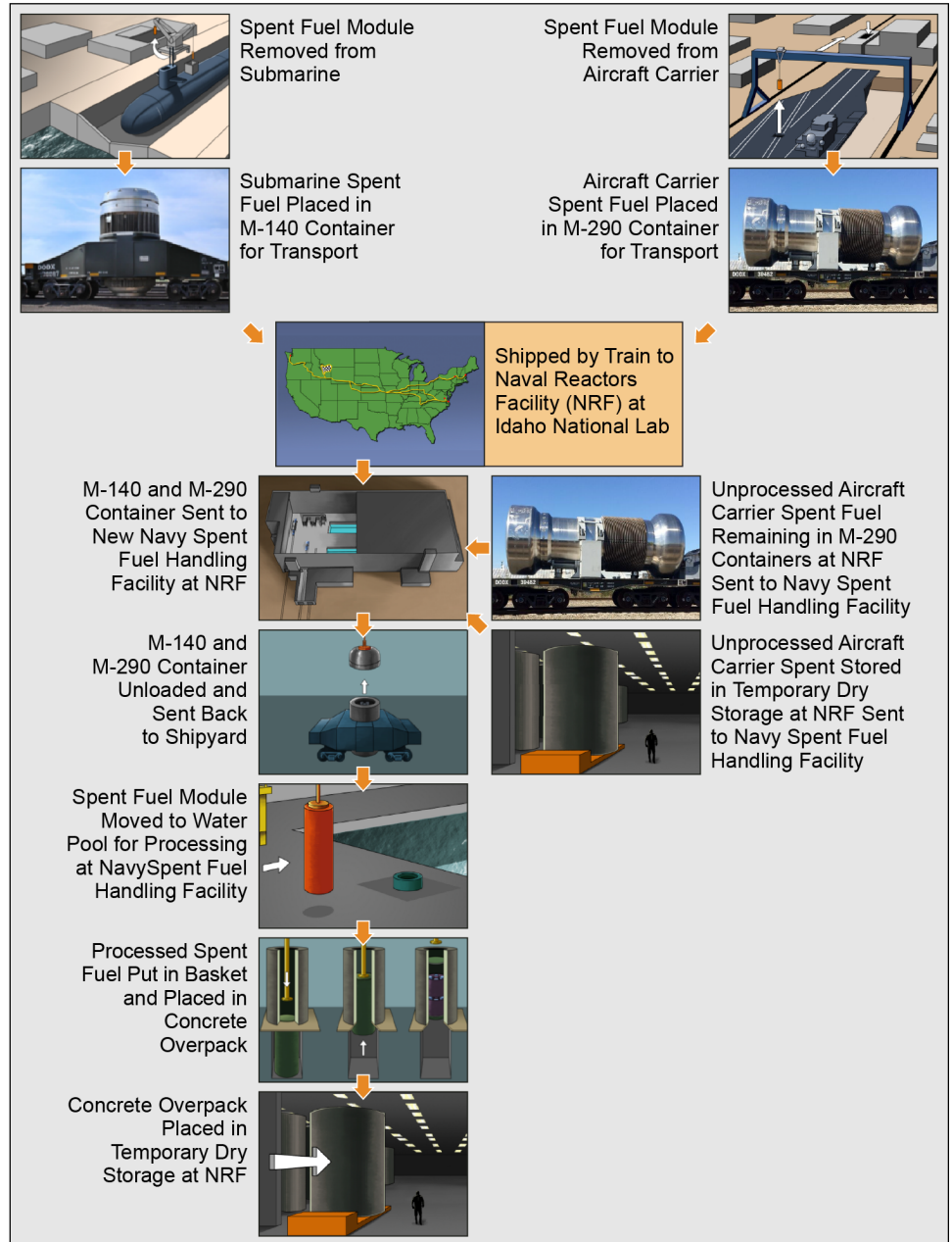
Figure 5: Future Process for Managing Naval Spent Fuel with the Spent Fuel Handling Facility
