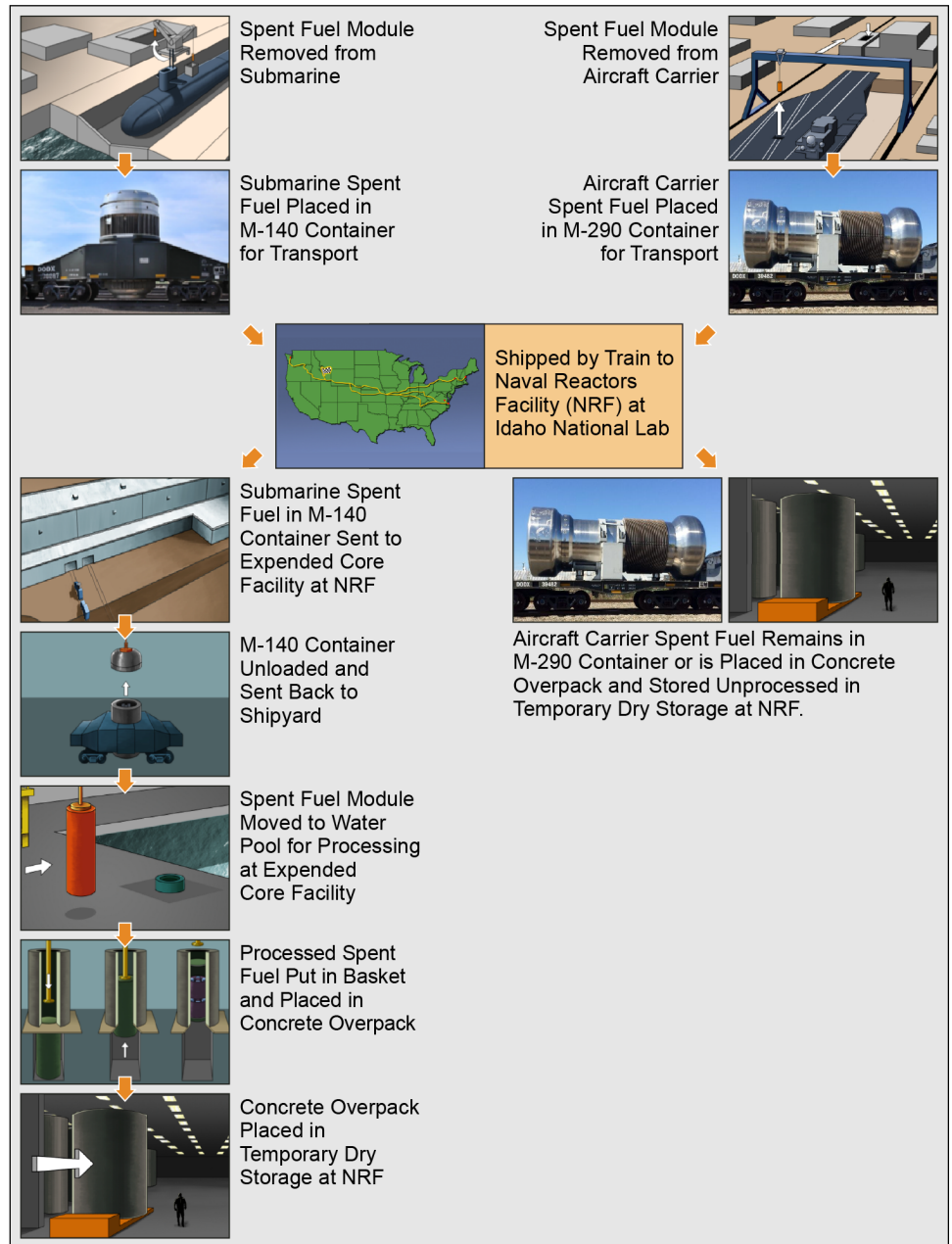
Figure 2: Current Process for Managing Naval Spent Fuel
