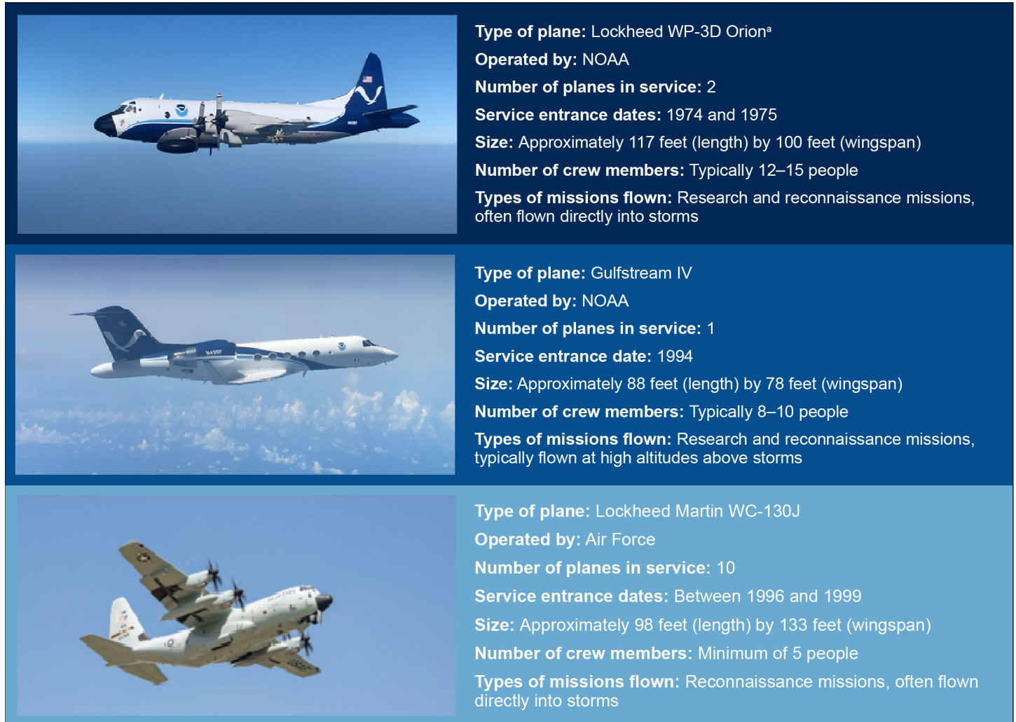
Figure 1: Overview of National Oceanic and Atmospheric Administration (NOAA) and Air Force Hurricane Hunter Aircraft
